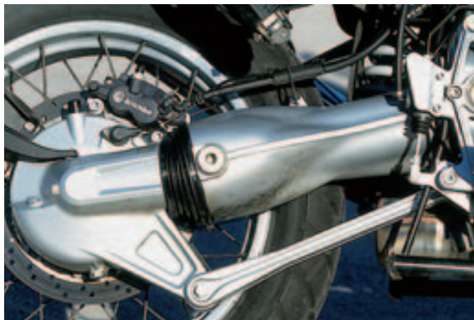
Pull the wheel back and problems might be revealed with oil leaking from the rubber cover
